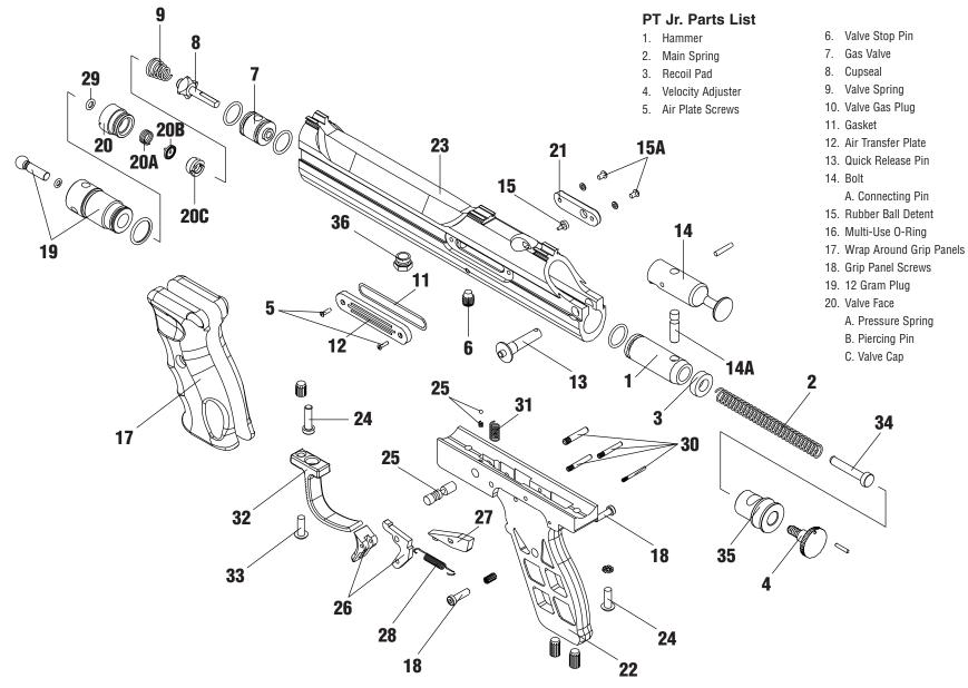
21. Ball Detent Cover 22. Grip Frame 23. Main Body 24. Grip Frame Screws 25. Safety Assembly 26. Trigger Plate 27. Sear 28. Sear Spring 29. Valve Face Seal O-Ring 30. Grip Frame Pin Set 31. Trigger Spring 32. Trigger Guard 33. Trigger Guard Screw 34. Spring Strut 35. Hammer Plug 36. Hex Nut
