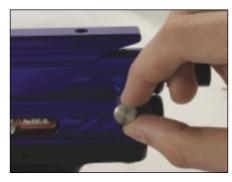
Figure 10. Remove field strip pin to begin disassembly.
