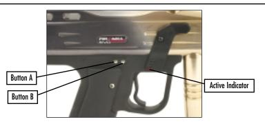
ANTI-CHOP EYE (ACE): When the ACE is activated, it will only allow you to fire when there is a paintball in the chamber. When the ACE is off, the rate of fire defaults to a slower setting so you won't chop paint. However, this means you will not be able to dry fire the marker quickly. To turn the ACE on or off, press button B on the right hand side of the frame while the marker is ready to fire. The Eye logo on the LCD will only appear while the ACE is turned on.
