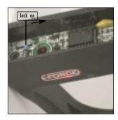
To access the Tournament Lock, you have to take the eForce frame off the receiver and unscrew the two phillips head screws (#13) that hold the board cover (#14) in place. Once these are out, the cover can be lifted and the small blue switch can be moved to put the marker on Tournament Lock.
