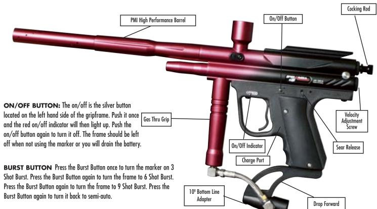
**SEAR RELEASE SLIDE**: The sear release slide is located on the left hand side of the Ravage grip frame. To reinstall the bolt/block/hammer assembly, push the sear release slide up before the hammer comes in contact with the sear. That will allow the bolt/block/hammer assembly to slide easily into the marker.
