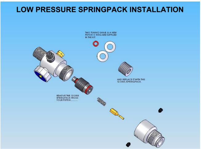
The installation of the of the Low Pressure Springpack is simple and requires only a 3/32" Allen wrench.
