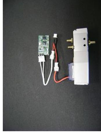
If you are not able to use one of the 3 supplied harnesses, it might be necessary to solder one of them to your marker. We recommend that you have Paintball Airmith solder the transmitter to your marker. It is possible to damage your marker/transmitter electronics, if not done properly.
