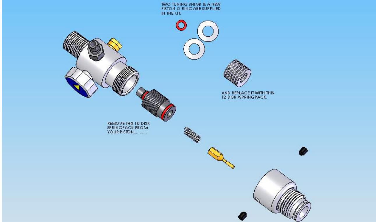
The installation of the of the Low Pressure Springpack is simple and requires only a 3/32" Allen wrench.
