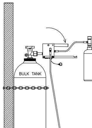
12. Unscrew the bottle from the fill adapter. Move Control Lever to the "Dump" position, and replace locking pin.
