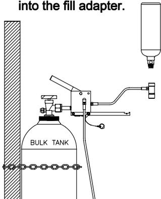
6. Turn the depressor knob on the fill adapter clockwise until it stops. Push the control lever to the DUMP position to drain the bottle completely.
