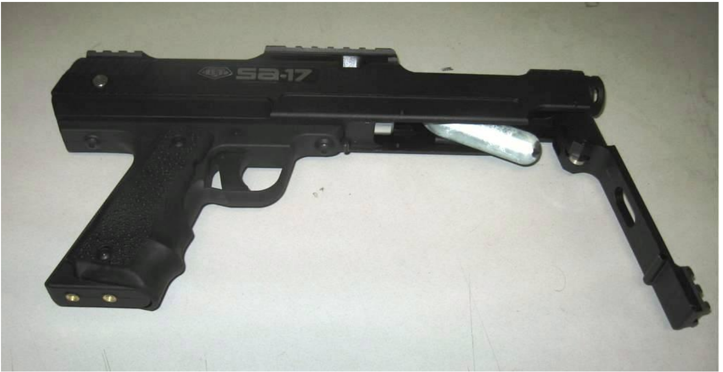
BT SA-17 paintball maker with lever to CO2 cartridge chamber open.
