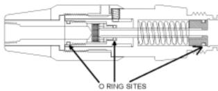
There are only three O-rings and one urethane Regulator seat in the EVIL® Detonator.™ If a leak is detected, the fault lies with one of the three O-rings. If the regulator fails to hold a consistent delivery pressure, then the problem is with the Regulator Seat (4).
