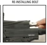
Line up with the back of marker so a sliver of the white bolt is showing & twist bolt 180° to lock back in place.
