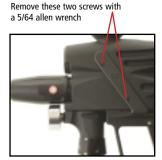
Replace worn or damaged ball detents
