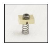
Screwing the Trigger Adjustment Screw (part #84) in further will make the spring push on the trigger more, and therefore make the trigger pull more stiff. Loosening the screw will make the trigger pull lighter. If you remove the plate, spring and screw the marker may bounce too much for tournament play. Make sure the cone of the spring is installed with the larger end down.
