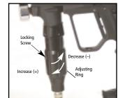
To adjust velocity, first loosen the locking screw (3/32 allen wrench) and back it off three full turns. If the locking screw is not backed off far enough you will be unable to turn the adjusting ring. The adjusting ring should turn easily; DO NOT FORCE IT!
