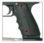
Unscrew the 2 clip bolts with a 5/32 allen key, or remove the 2 fieldstrip clip pins to release AEC frame.
