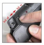
Turn on Tournament Lock by pushing the button up and turn it off by pushing the button down.
