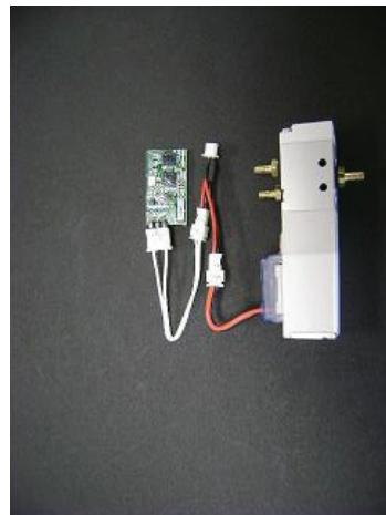
If you are not able to use one of the 3 supplied harnesses, it might be necessary to solder one of them to your marker. We recommend that you have Paintball Airsmith solder the transmitter to your marker. It is possible to damage your marker/transmitter electronics if not done properly.
