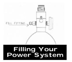
Your Reactor Preset Regulator is equipped with the standard "QD Style" fill fitting, which allows your system to be refilled either on or off the gun. Your Reactor Preset Regulator system may be filled with either <u>Clean, Dry</u> Compressed Air or Nitrogen. There will be no noticeable difference in your gun's performance.
